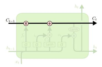
The LSTM does have the ability to remove or add information to the cell state, carefully regulated by structures called gates.
