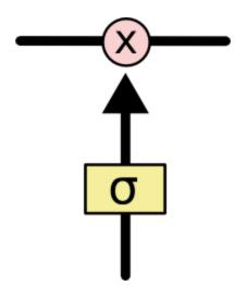
The sigmoid layer outputs numbers between zero and one, describing how much of each component should be let through. A value of zero means "let nothing through," while a value of one means "let everything through!"
