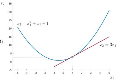
**Observation:** gradient of  $f(x_1, x_2)$  is parallel with the normal to the tangent of  $f(x_1, x_2) = 0$  at (3, 1).
