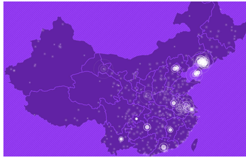
Fig. 20. A snapshot of detected FBSes in China at 19:00 on Jan. 16th, 2016, where each circle represents an active FBS.
