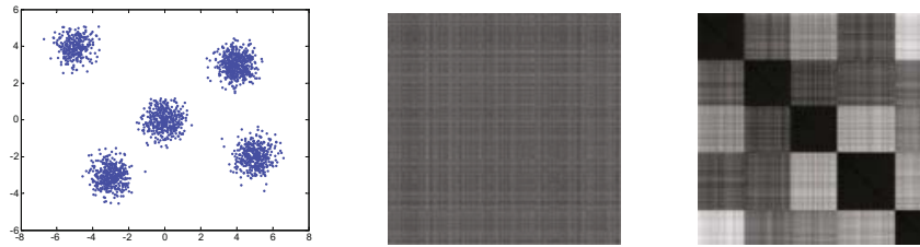
Figure 2.4: Data set, image from unordered objects and VAT image [BH02]. Lighter pixels correspond to larger distances, the dark squares along the diagonal correspond to dense regions in the data.
