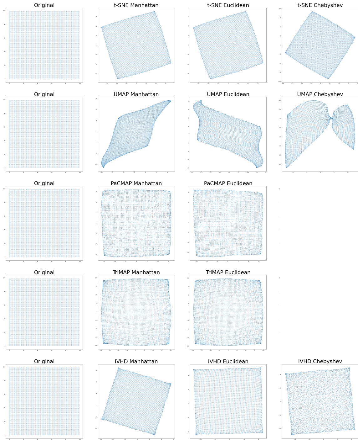
Figure 4.6: Methods comparison for embedding 2-dimensional grid using various metrics for calculating distance.
