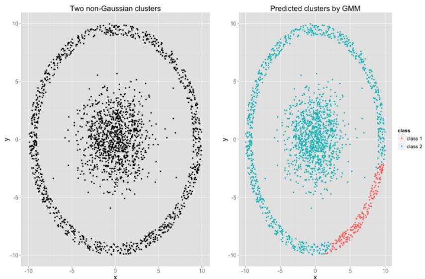
Fig.2: If data is not Gaussian, GMM clustering could not recognize right clusters
