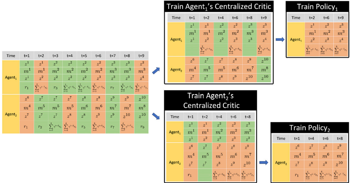
Figure 5. An example of the trajectory squeezing process in Mac-IAICC: each agent learns an individual centralized critic for the decentralized policy optimization. To better utilize centralized information, each agent's critic should receive all the valid joint macro-observation-action history (when any agent terminates its macro-action and obtains a new joint macro-observation). However, the critic's TD updates and the policy's updates still rely on each agent's individual macro-action termination and the accumulative reward at the corresponding time steps. Hence, the trajectory squeezing process for training each critic still depends on joint-macro-action termination but only retaining the accumulative rewards w.r.t. the corresponding agent's macro-action termination for computing the TD loss (the middle part in the above picture). Then, each agent's trajectory is further squeezed depending on its macro-action termination to update the decentralized policy.
